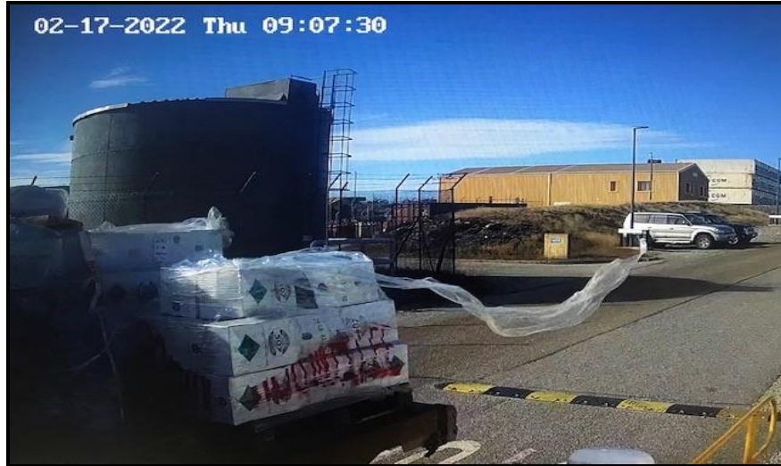
Fig 1: LGV Entering FIPASS with Insecure Load and Trailing Plastic.
